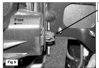
Use a pair of needle nose pliers to carefully pinch the top and bottom tab on the clip to release and remove the grille
