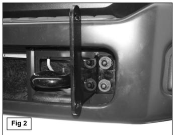
Before removing bumper bolts, measure gaps above bumper on driver and passenger side to relocate bumper
