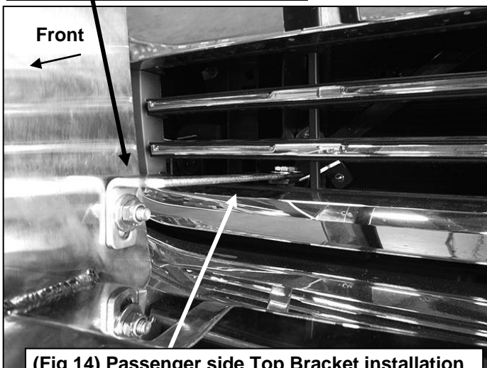
(Fig 14) Passenger side Top Bracket installation pictured. Adjust position so that Bracket cannot come in contact with plastic grille
