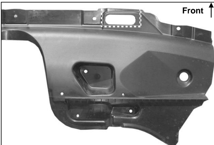
(Fig 23) Install and align the Grille Guard as per instructions. Tighten all hardware before marking the area on the splash guard to cut for clearance
