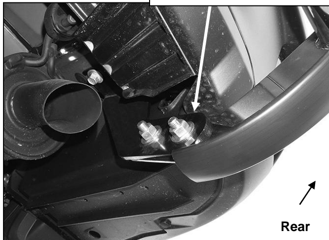
(Fig 7) Passenger side Frame Bracket installed
