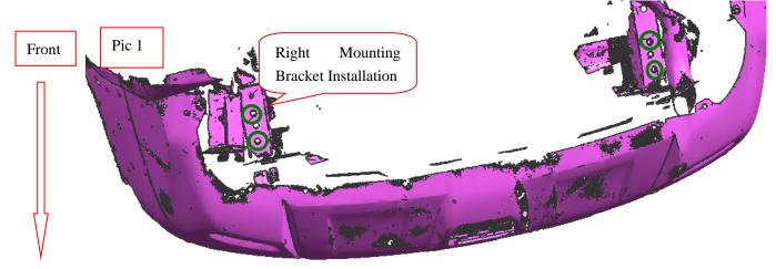
Step 3: Refer to the following picture to install the mounting brackets on the bottom but do not fasten.
