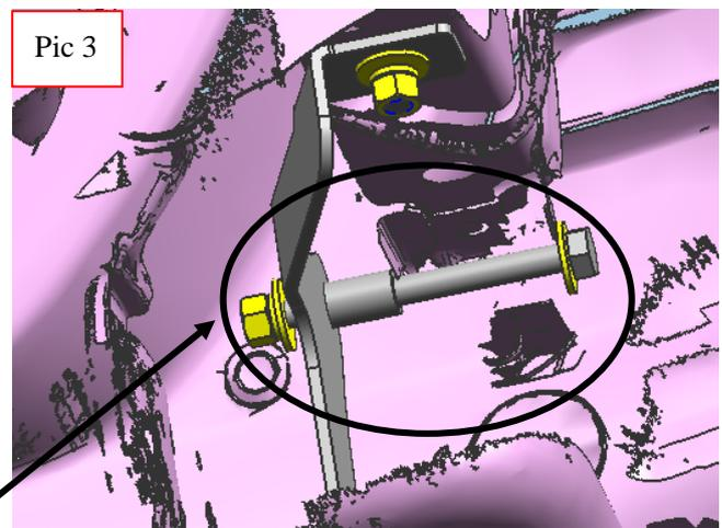
Step 3: Install the Rear Guard on the brackets and then adjust them to the proper positions.
