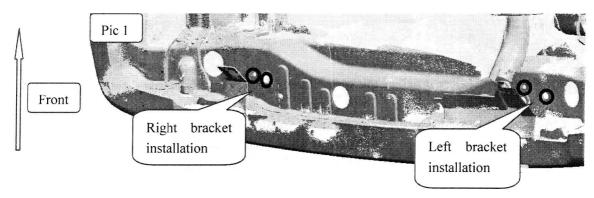
Step 3: Install the rear guard on the brackets and then adjust the brackets to the proper position.
