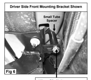
(10mm Clip Nut) 10mm x 100mm Hex Head Bolt 10mm Lock Washer 10mm Flat Washer
