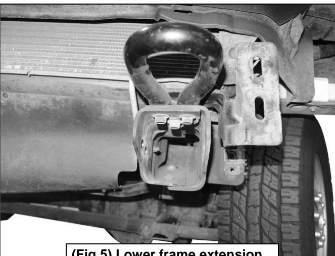
(Fig 5) Lower frame extension removed on driver side
