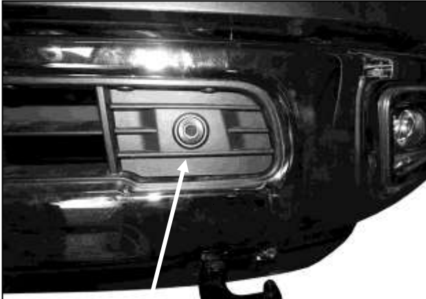
(Fig 1) Remove fill panel to access bumper bolts
