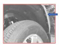
Install the short mounting bracket (RF1) into front of wheel well, using three factory fasteners and a T-15 Torx bit.
