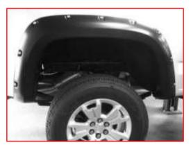
Holding flare in position, start five supplied Start three supplied screws (SW1-0056) into one forward and two rearward mounting holes.
