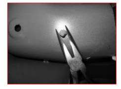
Once the factory fasteners have been removed, reach in behind deflector to find white factory retainer. Using pliers, pinch retainer and push towards wheel center, releasing deflector. Discard factory fasteners and deflector.
