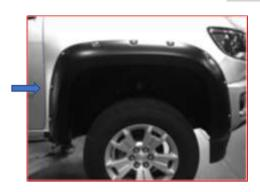
Using an awl, align clip with mounting hole and start one Pan Head screw. Do not tighten.
