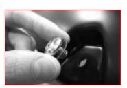
Put each Bolt/Washer combination through a pocket hole in the flare, Bolt head and Washer to the outside.
