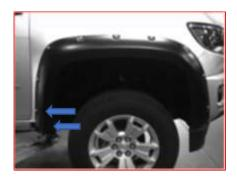
Start two supplied screws) into the two bottom rear mounting locations. Fully tighten all screws.
