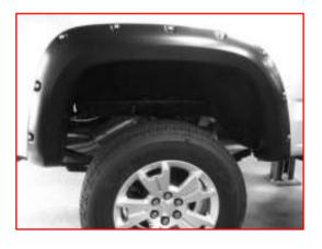
Fully tighten all screws. starting through the top center hole working outward. Use awl to align clip with mounting holes.
