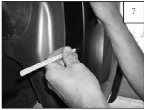
Holding flare in position on fender, use a grease pencil to mark the five clip locations.
