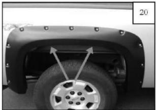
Reposition flare on fender. Start a supplied Screw (SW1-0058) through upper two hole locations and through each Clip (CL1-0022) installed in step 17. If needed, use awl to locate holes.
