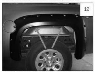
Reposition flare on fender. Start a supplied Screw (SW1-0058) through upper two hole locations and through each Clip (CL1-0022) installed in step 10. If needed, use awl to locate holes.
