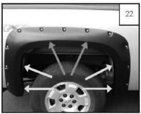
Fully tighten all screws starting with the newly installed Screws (SW1-0058) in upper two hole locations while pressing in on flare to ensure it is snug against sheet metal.
