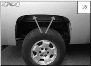
Slide a supplied Clip (CL1-0022) over top two factory holes. Clips may need to be adjusted to align with holes in flare. Note: Some vehicles with inner splash shelld will need to remove factory fasteners in indicated locations before installing the clips.
