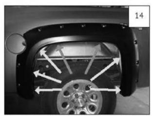
Fully tighten all screws starting with the newly installed Screws (SWI-0058) in upper two hole locations while pressing in on flare to ensure it is snug against sheet metal.
