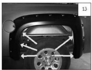
Start a supplied Screw (SW1-0050) through each of the remaining holes and into each Clip (CL1-0005) installed in step 11. If needed, use awl to locate holes.
