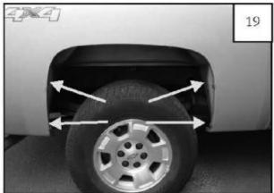
Slide a supplied Clip (CL1-0005) over lower four tabs. Clips may need to be adjusted to align with holes in flare.
