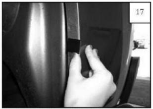
Center a supplied Tab (MT1-0002) over the marks made in step 15, aligning edge of tab with inside edge of fender lip (tab may extend over outside of fender).
