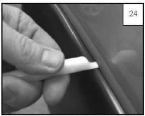
Using flat end of supplied Edge Trim Tool (ET1-0002), seat edge trim against flare by inserting straight end between edge trim and flare at one end. Next, slide around entire edge to the other end.
