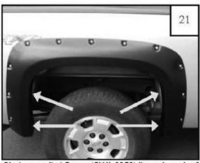
Start a supplied Screw (SW1-0050) through each of the remaining holes and into each Clip (CL1-0005) installed in step 18. If needed, use awl to locate holes.
