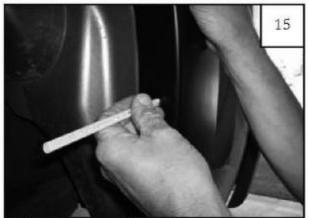
Holding flare in position on fender, use a grease pencil to mark the four clip locations.
