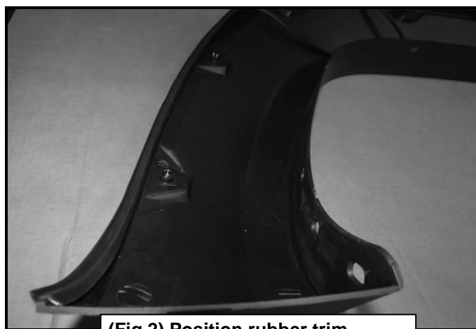
(Fig 2) Position rubber trim correctly with the wiper side on the outer surface of the flare
