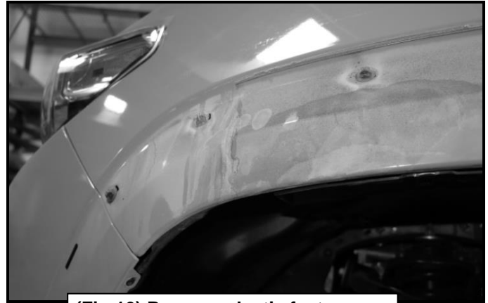
(Fig 10) Remove plastic fasteners
