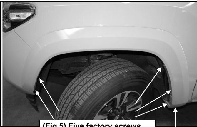
(Fig 5) Five factory screws, driver's side front
