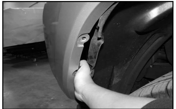
(Fig 8) Insert hand behind this section to release hidden fasteners
