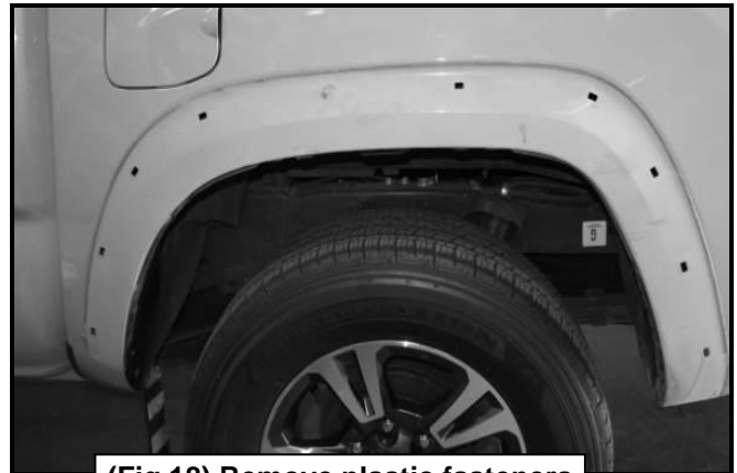
(Fig 18) Remove plastic fasteners
