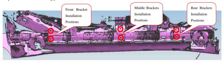
Step 3: Install the side bar on the brackets and then adjust the side bar to the proper positions.
