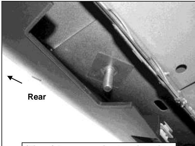
(Fig 17) Rear mounting location with Bolt Plate pictured from below
