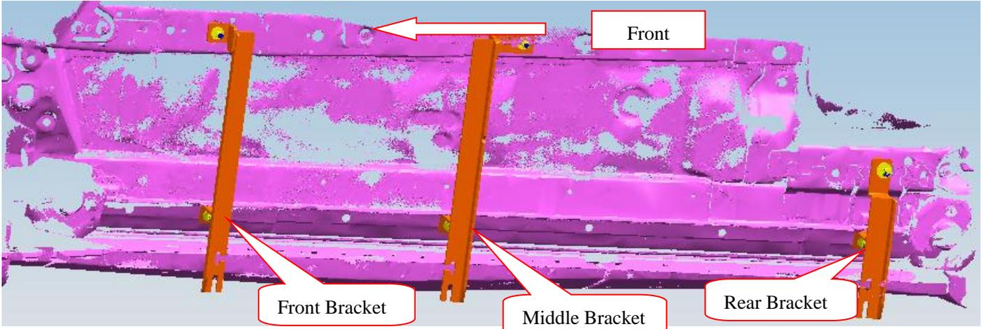
Step 3: Install the running board on the brackets and then adjust them to the proper positions.
