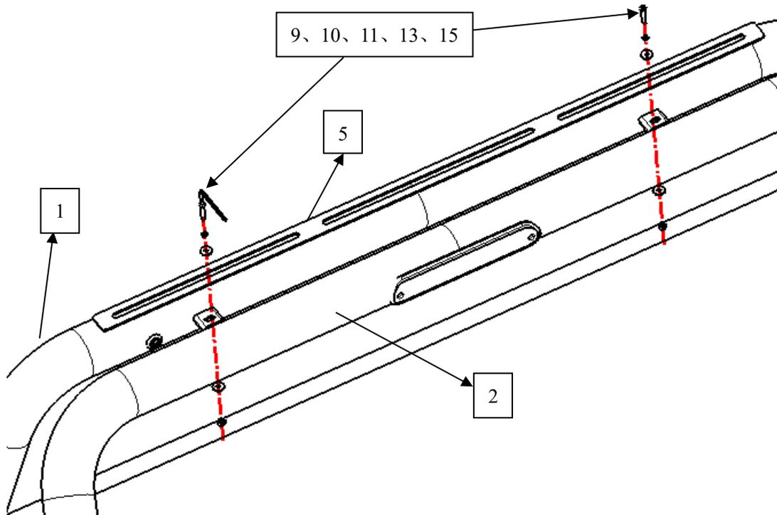
Step 3: Using wrench 14, install 3/4 decoration plate together with parts 19/20/21/24 as shown.
