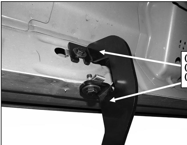
(Fig 7) Driver/left rear bracket installed
