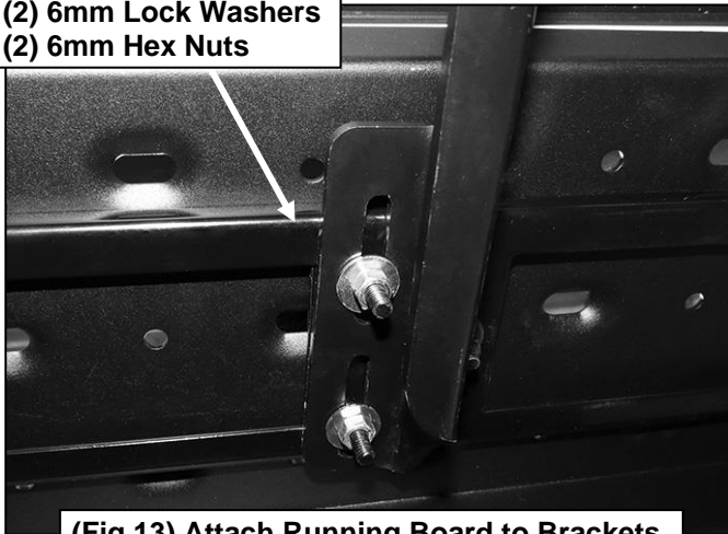
(Fig 13) Attach Running Board to Brackets
