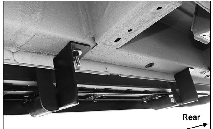
(Fig 22) Passenger side center and rear Brackets installed-mark to drill through pinch weld
