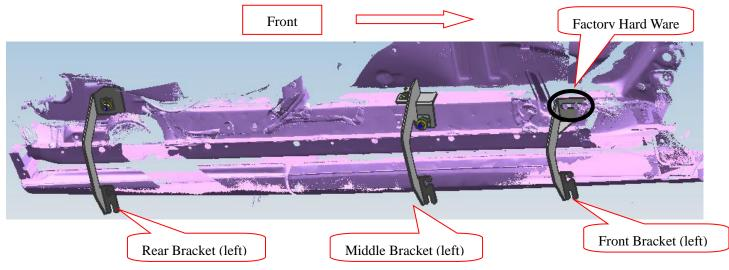
Step 3: Install the running board on the brackets and then adjust them to the proper positions. Step 4: Check if all hard ware are installed and then fasten all to complete the installation.
