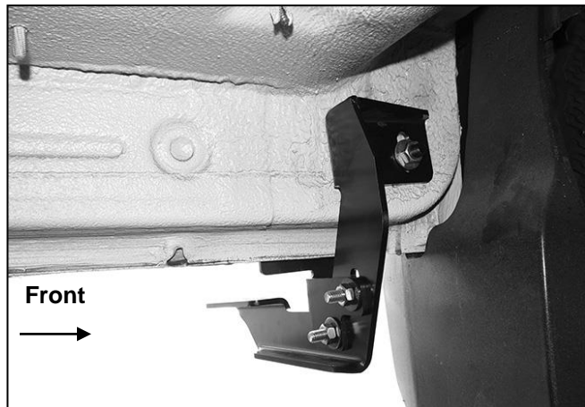
(Fig 19) Driver/left Front Bracket pictured (Note driver side front and rear Brackets are identical)
