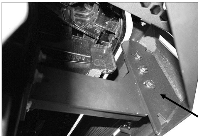
(Fig 10) Passenger/right side of Bumper attached to Bumper Bracket (pictured from below)
