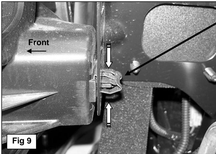
Use a pair of needle nose pliers to carefully pinch the top and bottom tab on the clip to release and remove the grille
