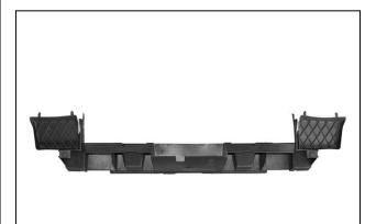
(Fig 5A) 2011-13 Models: Inner air deflector assembly-applies to vehicles without tow hooks
