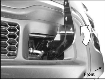
(Fig 11B) Rotate the Bracket to meet the mounting holes for the tow hooks
