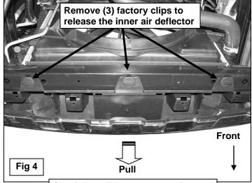
Carefully pull bumper cover forward and remove inner air deflector
