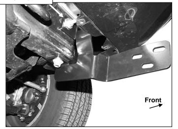
(Fig 6) Driver side Frame Bracket installed
