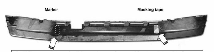
(Fig 15) Use removable tape (masking tape) or a marker to mark location of Frame Brackets onto back of air dam (arrows). Carefully cut small openings with a sharp knife or hacksaw blade.
