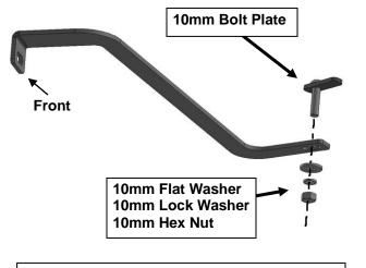
(Fig 11) Passenger side Top Support Bracket
