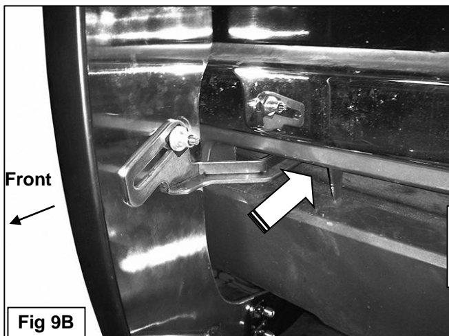
(Fig 8B) Install Frame Bracket with factory tow hook bolts. Small tow hook pictured
