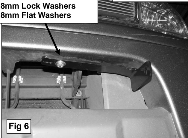
05-08 driver side Top Bracket installation pictured
