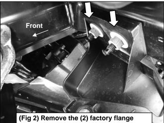
nuts, per side, to remove active air dam
