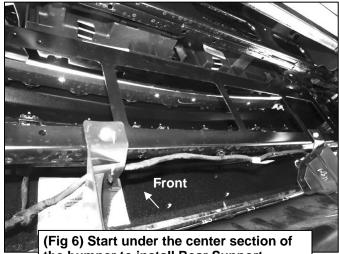
the bumper to install Rear Support Bracket, (Pictured from behind bumper) IMPORTANT: Installing the Rear Support Brackets will require multiple movements of the Bracket to get to the mounting location.
