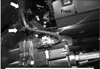
(Fig 1) Unplug and release the harness from the plastic clips to remove active air dam
