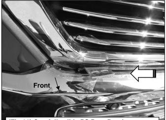
(Fig 11) Carefully slide PS Rear Bracket towards the passenger/right side of the vehicle
