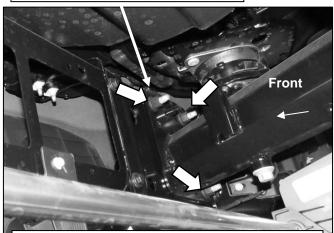
(Fig 4) IMPORTANT: DO NOT remove bumper, ONLY slightly loosen bumper to install Support Brackets. (Passenger/right side frame pictured)
