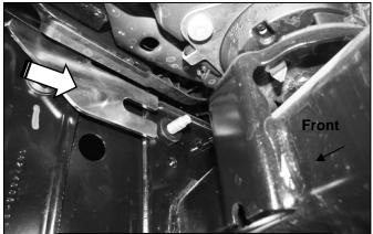
(Fig 12) Place (1) 12mm x 29mm Spacer Washer over the stud in the frame. Slide the Bracket over Washer
