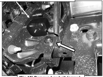
(Fig 10) Remove hex bolt (arrow)
