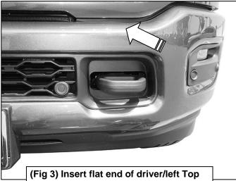
(Fig 3) Insert flat end of driver/left Top Bracket through bumper (arrow)
