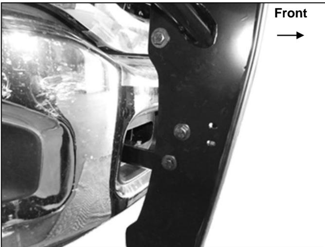
**(Fig 15) Attach Grill Guard to outside of Mounting Brackets (passenger/right side pictured)**
