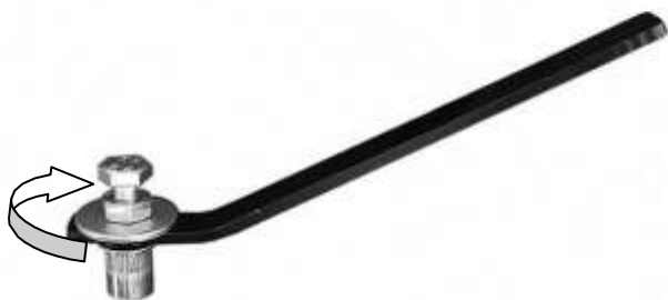
(Fig 5B) Assemble 6mm Insert Tool
