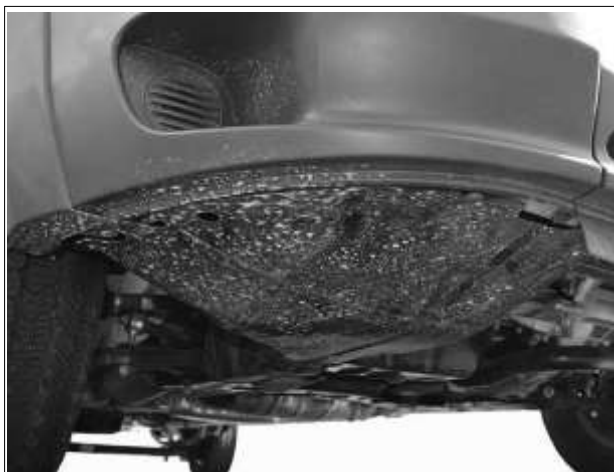
(Fig 1) Remove plastic splash guard.
