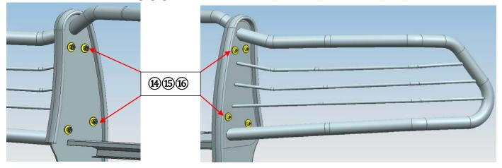
Step 2: Remove tow hook. Use standard parts 0 1 1 1 1 2 3 to install bracket L/R on the original mounting points of tow hook.
