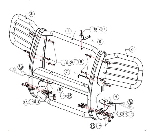
Step 1: Install left and right brush guard on the front guard.
