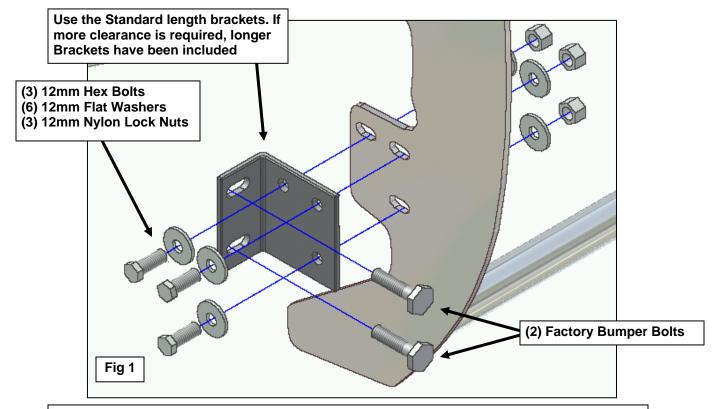
**WARNING!** Do not remove passenger and driver bumper bolts at the same time or bumper may fall. Only remove and install one Frame Mounting Bracket at a time.
