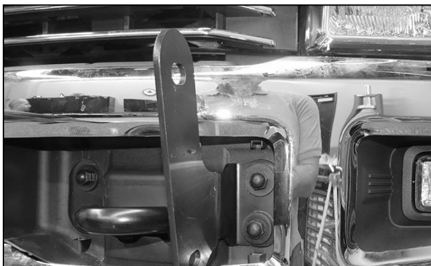
(Fig 5) Reuse factory bumper bolts to attach driver/left Frame Bracket to Spacer and bumper
