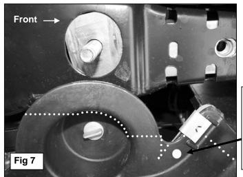
Move metal clip to here (Dot) or drill a 1/4" hole and replace the clip with the included:
