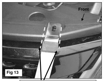
Place Top Bracket in mounting position. Mark removable tape on plastic cover as required to clear Top Bracket
