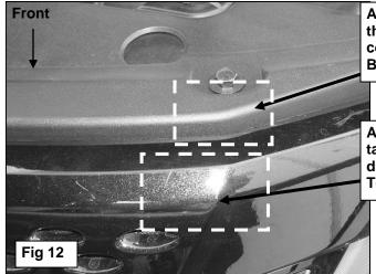
Apply a layer of removable tape to this area to mark (or mark back of cover) before cutting for Top Bracket installation (Fig 15 & 16)
