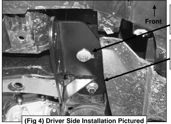
12mm x 50mm Hex Bolt 12mm Lock Washer 12mm Flat Washer
