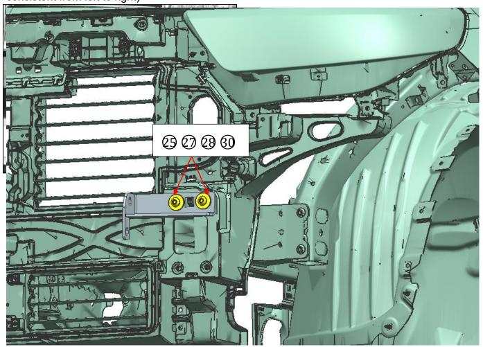
Then connect Bottom Support Brackets to Upper Brackets with standard parts 19 20 20 .
