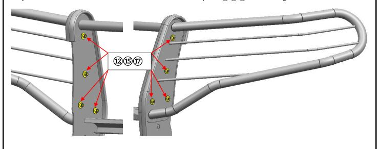
Step 2: Remove the original plastic front bumper. Fix the Bottom Support Brackets with standard parts 25 27
