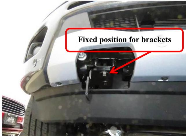
Step 4: Connect Step 2 grille guard with the brackets. Align the Grille Guard properly and tighten all hardware.
