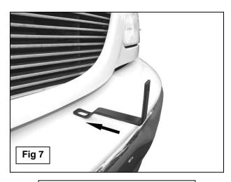
Insert Top Mounting Bracket between grille and top of bumper
