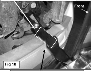
Protect the top of the plastic bumper cover with masking tape to prevent scratches during installation
