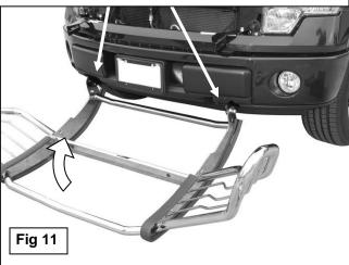
Insert 12mm Plastic Washers between the Grille Guard and the Mounting Bracket. Line up the holes in the Plastic Washers with the mounting holes. Insert the Mounting Bolts through the Plastic Washers
