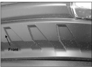
(Fig 4) Example of lower bumper cover on vehicles without tow hooks
