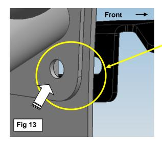
Put one Hex bolt M10\_35 & one Flat washer D10(10x30x2.5mm) between the guard and bracket.
