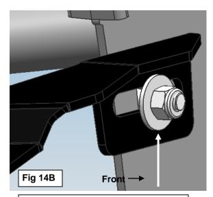
Hexagon jam nut M10& Flat D10(10x30x2.5mm). Tighten all the bolts.
