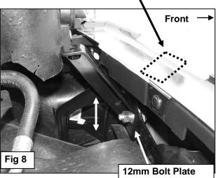
12mm Lock Washer 12mm Flat Washer 12mm Hex Nut
