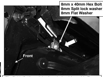
(Fig 5) 2015-17 models: Attach the driver side Top Bracket to the middle mounting hole on the top of the bumper bracket (pictured from behind bumper)
