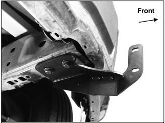
(Fig 16) Attach Frame Bracket to Nut Plate.
