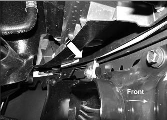
(Fig 6) 2015-17 models: Attach the driver side Top Bracket to the middle mounting hole on the top of the bumper bracket (pictured from behind center of bumper)
