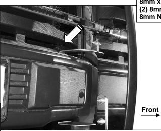
8mm x 30mm Hex Bolt (2) 8mm Flat Washers 8mm Nylon Lock Nut
