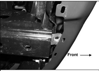
(Fig 13) Insert Nut Plate into open end of frameapplies to models without tow hooks only
