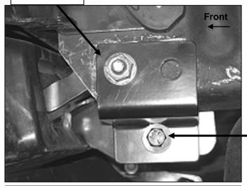
(Fig 7) Passenger side Support Bracket bolted to inside of frame and pictured from behind bumper
