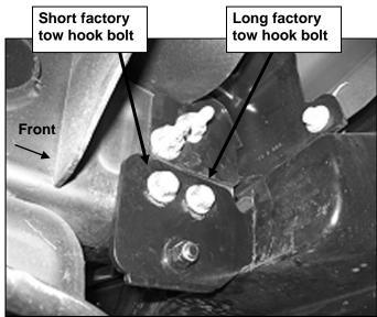
(Fig 6) Passenger side Mounting Bracket bolted to outside of frame and pictured from behind bumper
