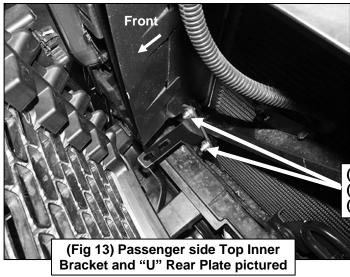
Remove hardware securing grille to vehicle. Carefully pull the grille straight out from the vehicle. Tilt the top of the grille forward only to access the area behind the grille
