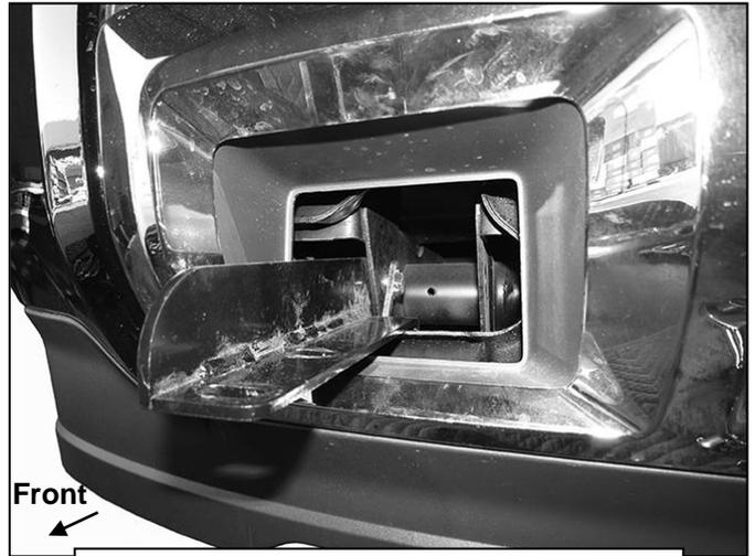
(Fig 6A) Passenger/right Frame Bracket
