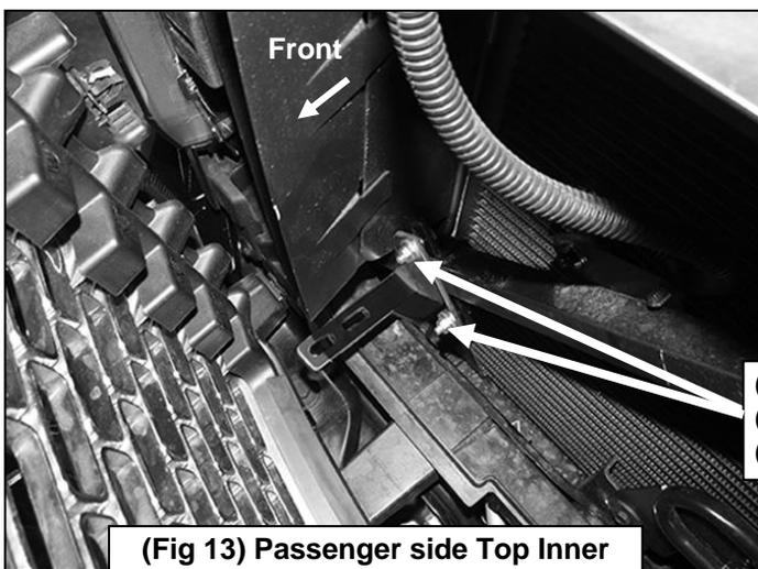
(Fig 13) Passenger side Top Inner Bracket and "U" Rear Plate pictured
