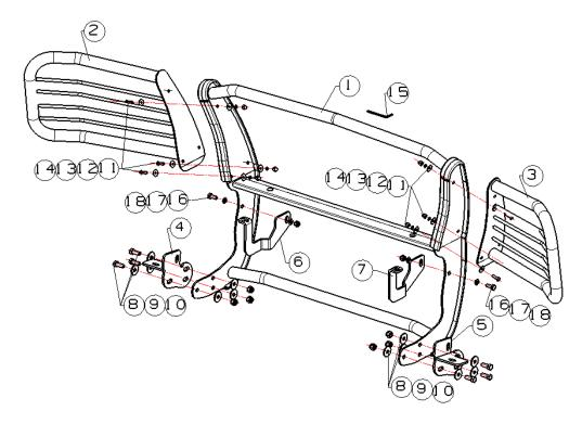
Step 1:Install two brush guards on the front guard.
