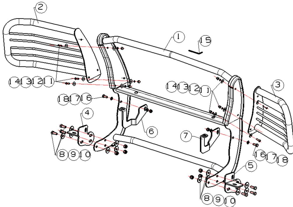
Step 1: Install two brush guards on the front guard.
