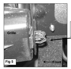
Close up view of retaining clip on back of grille insert
