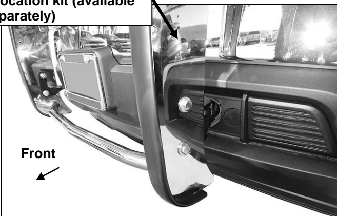
(Fig 19) Attach Grille Guard to Mounting Brackets
