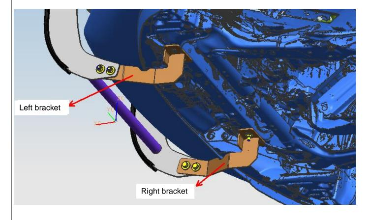
B. Open the engine cover, install left and right support brackets with factory bolts as figure 3. Snug but do not tighten hardware.
